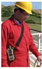
MultiRAE used for worker exposure monitoring at an oil refinery
