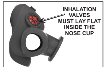
FIGURE 2 CHECK INHALATION VALVES ON THE IMD NOSE CUP
