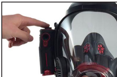
FIGURE 25 TURN ON THE TIC
