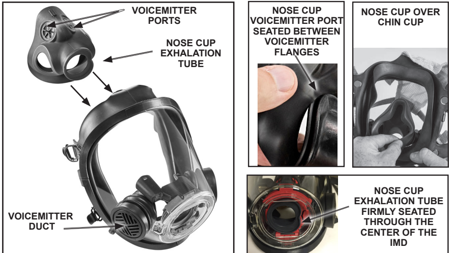
FIGURE 19 INSTALLING THE NOSE CUP
