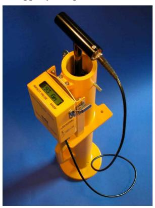
Introduction: - The 4.5 Kg CIST/883 Clegg Impact Soil Tester manufactured by SDi provides an easy and straightforward means for measuring and controlling soil strength and consolidation levels during trench re-instatement. The 883 readout is clamped to the guide tube and the displayed reading is viewed from the top during use. Single button operation design provided for easy use.
