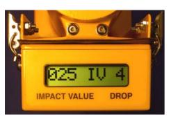
The Readout Unit displays readings of Impact Value (IV) and also shows the number of times that the hammer has been dropped during each test operation. Example:- readings of 25 IV and drop number 4 are shown on the readout unit in the picture on the left.
