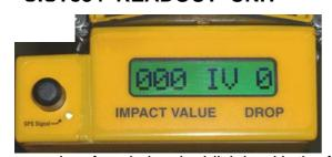
The Readout Unit displays readings of Impact Value (IV) and also shows the number of times that the hammer has been dropped during each test operation. The number of GPS satellites detected is also displayed confirming successful GPS location fixes.
