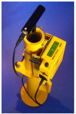
Introduction: - The GPS equipped 4.5 Kg CIST/884 Clegg Impact Soil Tester manufactured by SDi provides an easy and straightforward means for measuring and controlling soil strength consolidation levels during trench re-instatement. The GPS 884 readout is clamped to the guide tube and the displayed reading is viewed from the top during use. Single button operation design provided for easy use.
