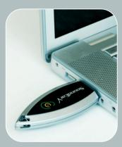
SoundEarV enables each member of staff to receive a message when the pre-set noise level is exceeded – a pop-up function warns against the fact that the noise limit has been exceeded – without disturbing the work being done on the computer at the time.
