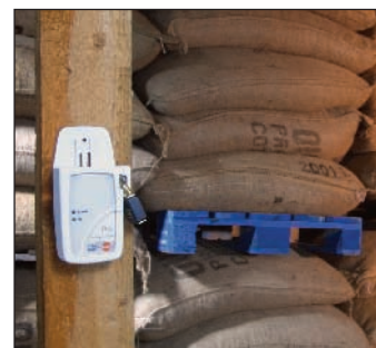
Monitors humidity and temperature values e.g. in warehouses
