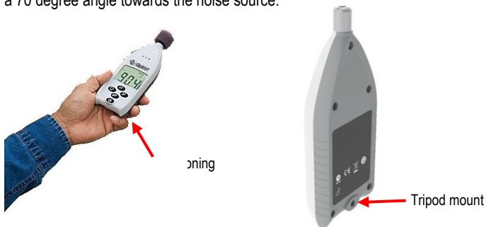
Figure 1-9: Positioning and tripod mount
