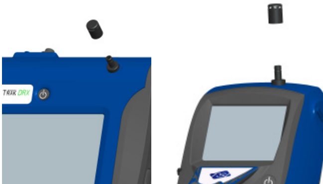
Figure 2-3: Putting on Inlet Cap
