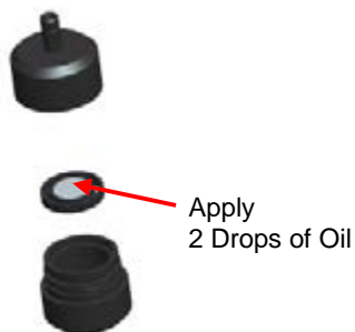
Figure 4-4: Apply 2 Drops of Oil to Impactor Plate
