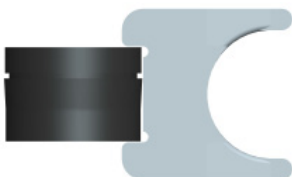
Figure 4-20: Replace Mesh in Filter Holder
