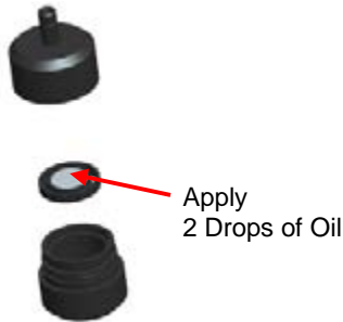
Figure 4-4: Apply 2 Drops of Oil to Impactor Plate
