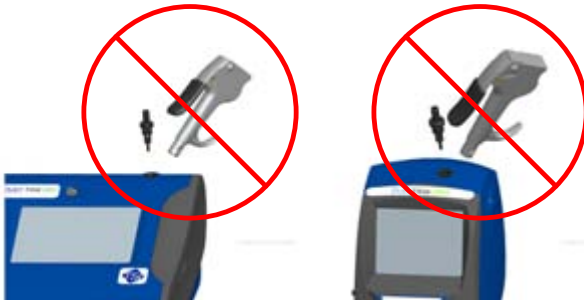
Figure 4-3: Do NOT Blow into Instrument
