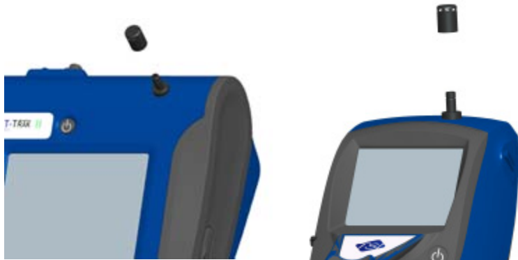
Figure 2-3: Putting on Inlet Cap
