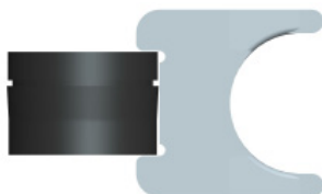
Figure 4-10: Replace Mesh in Filter Holder
