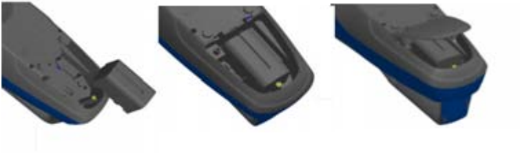
Figure 2–2: Batteries into Handheld Unit
