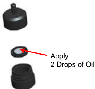
Figure 4-4: Apply 2 Drops of Oil to Impactor Plate
