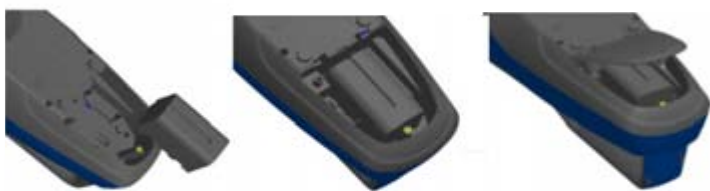
Figure 2–2: Batteries into Handheld Unit
