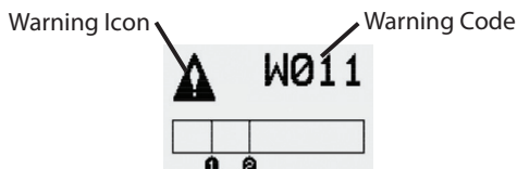
Figure 32. General Status Warning - detail
