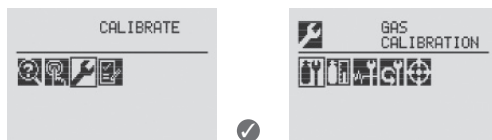
Figure 41. Gas Calibration menu
