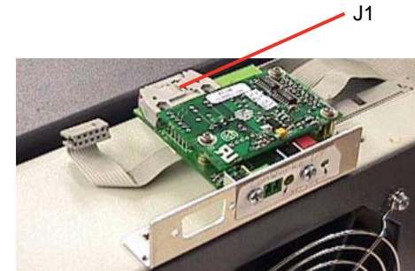
Figure G-6. Ribbon Cable Connected to J1 (Rack Mount Units)
