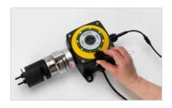
The box is configured using a magnetic switch. A magnet is incorporated into the blanking cap which screws into the middle of the box lid when not in use. The following parameters can be configured: -
