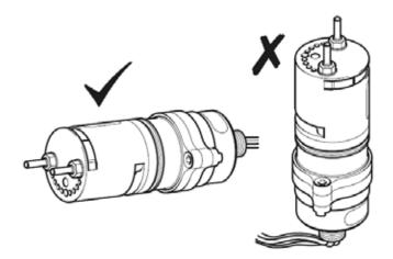
3) Secure the junction box onto the mounting surface, using the Junction Box Adaptor Plate if required. Searchpoint Optima Plus must be installed with its long axis horizontal in order for the standard weather protection to operate correctly and to prevent water from settling on the optical surfaces (see below). The Optima unit should therefore only be screwed into a threaded entry that is in a vertical wall of the junction box. The deluge/heat shade (supplied as standard) should also be fitted.
