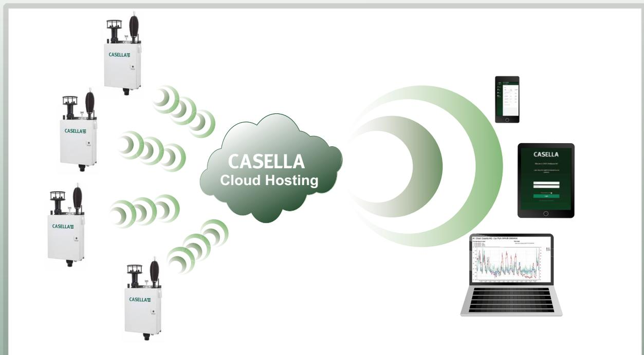
The Guardian2 advanced mHub datalogger and web connectivity allows data to be continuously sent to the cloud. Alerts and status reports can be seamlessly delivered to your mobile device.
