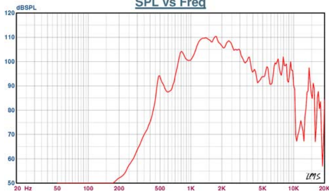
Sound pressure levels at 1W/1m 28mm
