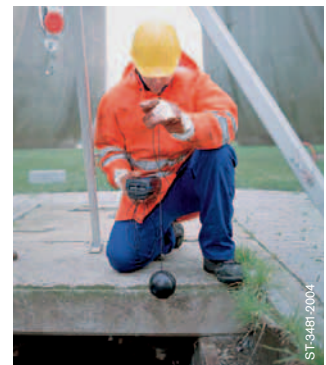
Dräger CMS with Remote-System: Measurement with extension hoses of up to 10 m in length.
