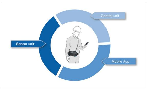
The Dräger X-pid® 9000/9500 consists of three elements: You control the sensor unit via the control unit and the pre-installed mobile app. The sensor unit can be worn around the neck, keeping one hand free.
