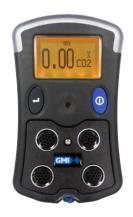
The PS500-CO2 detects 0-5% volume CO<sub>2</sub> reliably and accurately using infrared capabilities.
