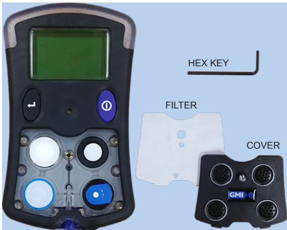
Fig. 4.2 Filter and Cover Removed
