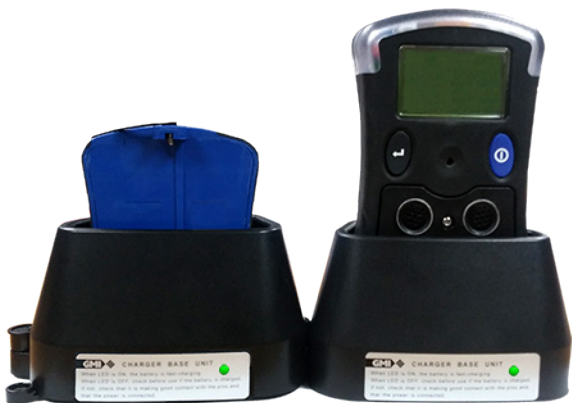
Fig. 4.9 Battery Pack / Instrument 'Docked' in Fast Charger / Slave Unit(s)
