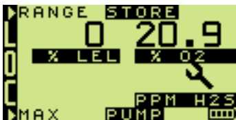
Fig. 4-10 H2S Sensor Fault
