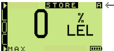
Fig. 3-34 Alarm Enabled Identifier
