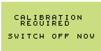
Fig. 4-12 Calibration / Configuration Memory Fault
