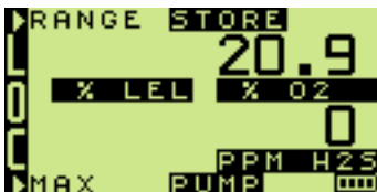
Fig. 3-30 Faulty Range Display
