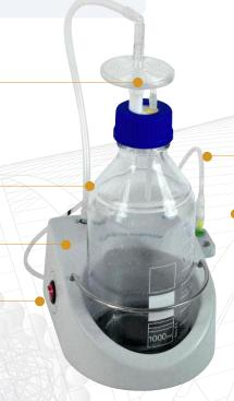
1L trap flask for collection of alcohol/buffer from microtest tube walls during reprecipitation
