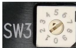
Figure 3-3 SW3 Ten (10) Position Rotary Switch
