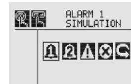
Figure 16. Alarm/Fault Simulation Menu
