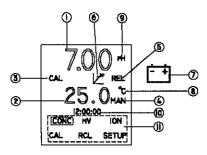
1. Primary display - provides direct readout of pH, Activity, mV or Ion samples.
