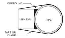
Over time temporary coupling compounds (e.g. Petroleum Gel) may gradually sag away from the sensor resulting in reduced signal strength and finally complete loss of signal. Warm temperatures, moisture and vibration will accelerate this process. Dow Corning Silicone Compound #4 as supplied with the UF D5000 (and available from Micronics Limited) is recommended for semi-permanent installations.
