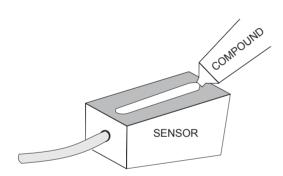
Use the PC4 pipe clamp (supplied) as illustrated above or use a loop of electrical tape for temporary mounting. Apply silicon coupling compound #4 to the coloured face of the sensor. A bead, similar to toothpaste on a toothbrush, is ideal. Do not overtighten (crush the sensor).
