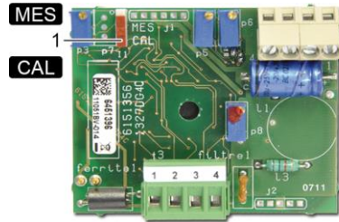
Figure 15: CTX 300 SC main circuit board.
