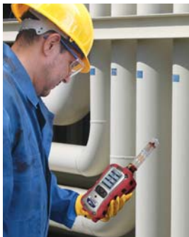
Multi RAE Benzene used for leak detection
