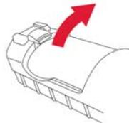
4. Replace a fully charged spare battery pack inside the battery compartment. Make sure the battery pack is oriented properly inside the compartment.
