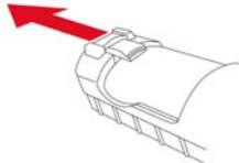
3. Remove the battery pack from the battery compartment by tilting it out.
