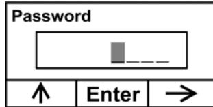
2. You do not need a password to perform calibrations. Instead of inputting a password, enter calibration by pressing [MODE].
