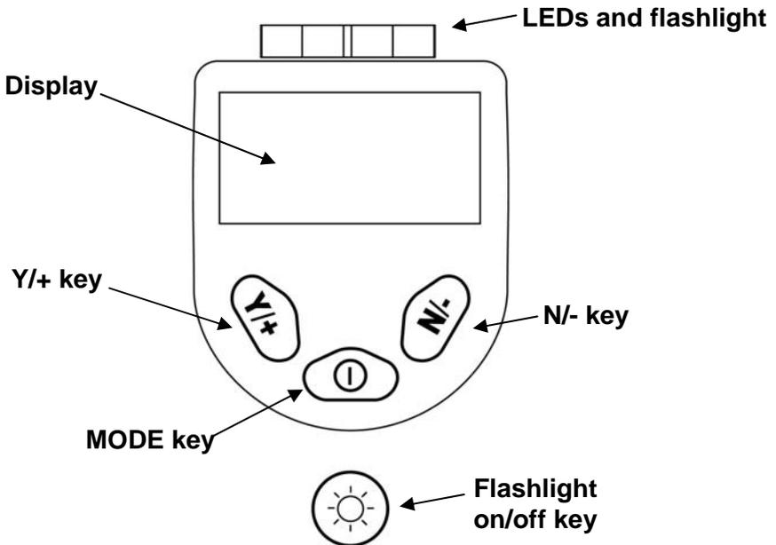
In addition to their labeled functions, the keys labeled Y/+, MODE, and N/- act as “soft keys” that control different parameters and make different selections within the instrument's menus. From menu to
