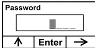
2. You do not need a password to perform calibrations. Instead of inputting a password, enter calibration by pressing [MODE].
