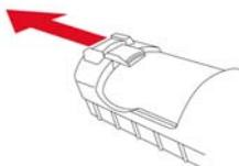
3. Remove the battery pack from the battery compartment by tilting it out.
