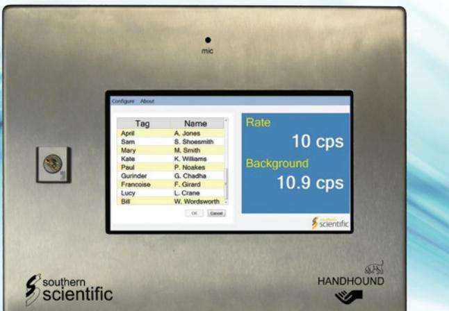
not in use. A proximity sensor ensures the user's hands are underneath the detector, the user then speaks his/her name and says 'Continue'. The system will begin counting for a predetermined period, set by the supervisor. A touchscreen interface is also incorporated, to allow configuration and manual triggering if needed.
