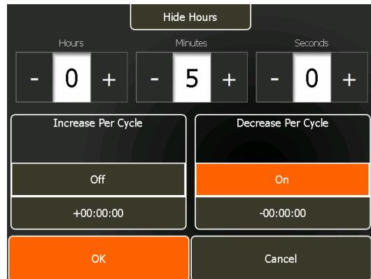
A new screen will open which is similar to the simple time entry screen. The maximum decrease in hold time per cycle (based on the number of cycles and the time limits of the unit) will be shown.
