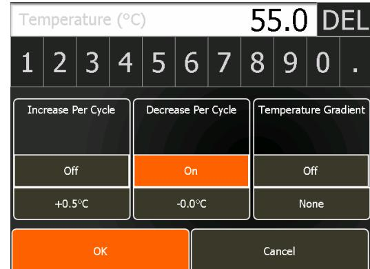
A new screen will open which is similar to the simple temperature entry screen. The maximum decrease in temperature per cycle (based on the number of cycles and the temperature limits of the unit) will be shown.
