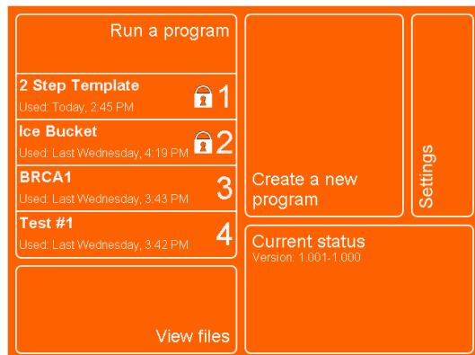
If there is one or more Satellite unit(s) connected to the TC-PLUS, an additional screen will ask if you wish to run the program on a selected Satellite unit or the TC-PLUS
