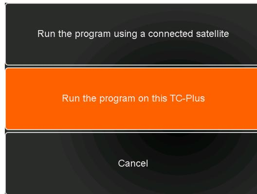
If it is decided to run the program on a Satellite unit, an additional screen will allow selection of the required unit.
