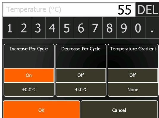
A new screen will open which is similar to the simple temperature entry screen. The maximum increase in temperature per cycle (based on the number of cycles and the temperature limits of the unit) will be shown.
