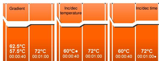
If a step has an incremented or decremented temperature, this will be indicated by a white spot next to the temperature.
