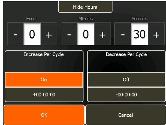
A new screen will open which is similar to the simple time entry screen. The maximum increase in hold time per cycle (based on the number of cycles and the time limits of the unit) will be shown.
