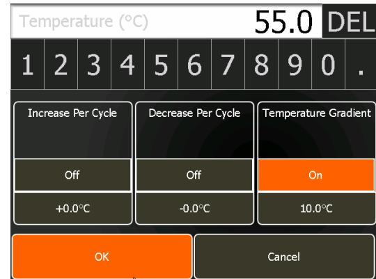
The temperature value will now appear orange in the programming screen indicating that it contains a modified function.
