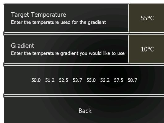
**Note:** With the 384-well block, the columns are paired as it is not possible to individually control 24 columns. Therefore only 12 column temperatures are available across this block.
