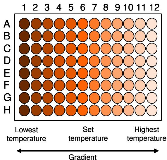
The maximum temperature gradient range which can be set is 30°C and the minimum is 1°C; the lowest temperature is 0°C or 20°C below ambient and the hottest temperature is 100°C. Examples are given in the table below:
