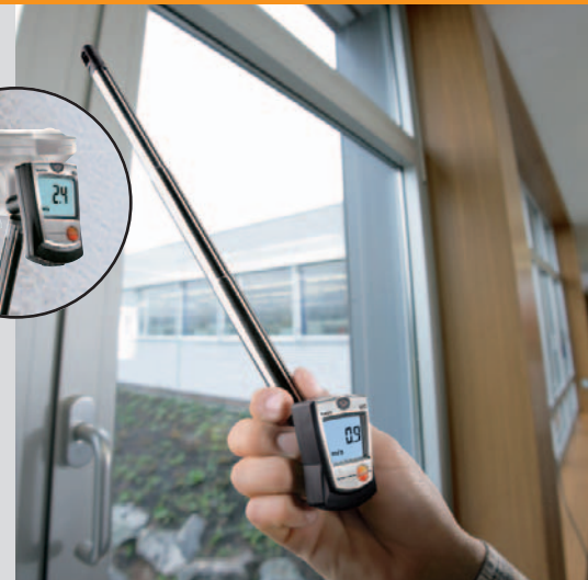
Flow velocity measurement at nontight windows
