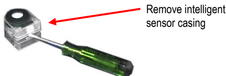
Figure 7-2: Removing intelligent-sensor casing with PID
