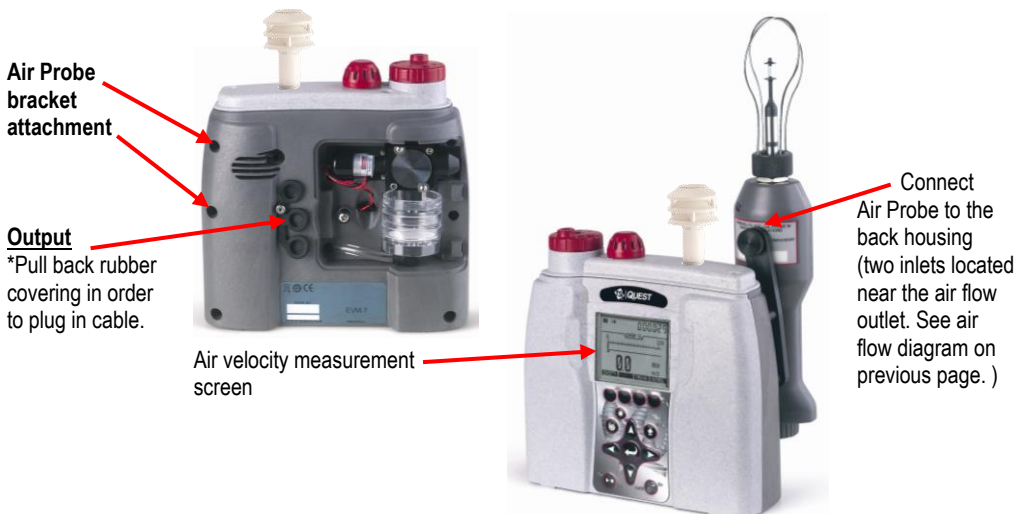
Figure 5-11: Attaching Air Probe and measuring Air velocity
