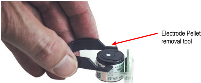
Figure 7-3: Removing the lamp with removal tool
