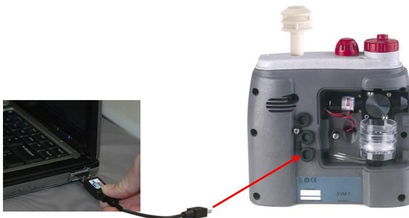
Figure 2-7: Communicating with DMS via USB cable
