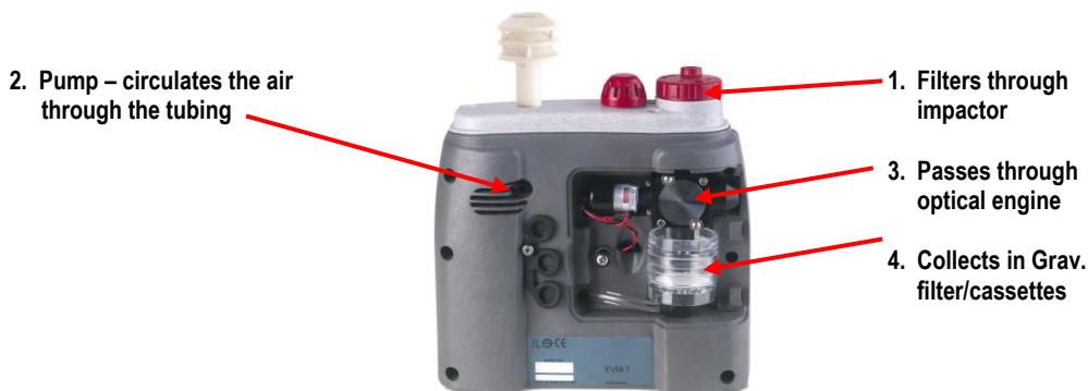
Figure 4-3: How the impactor functions
