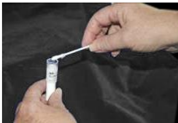
Figure 7-5: PID sensor cleaning kit (optional accessory)
