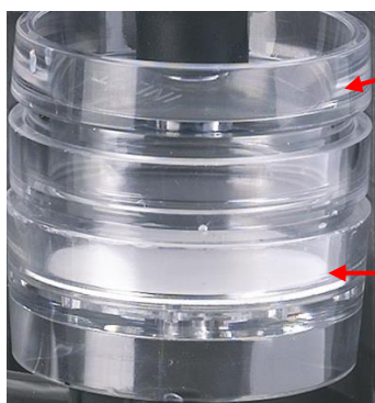
Figure 7-10: Gravimetric cassette and filter paper maintenance
