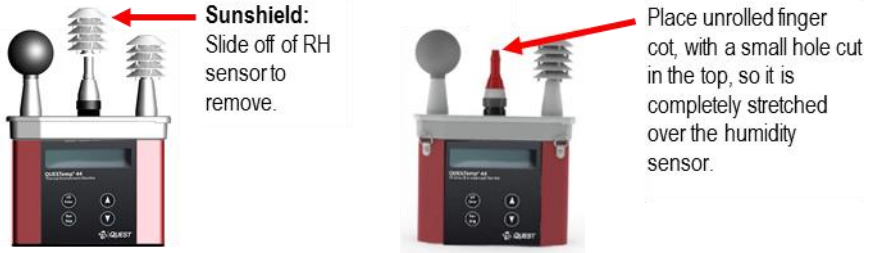
Figure 1-22: Sunshield & placement of finger cot prior to RH verification
