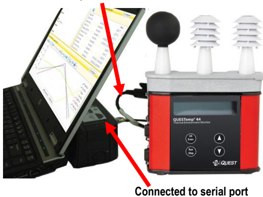
Figure 1-30: Communicating with the QT o 44/46 and DMS
