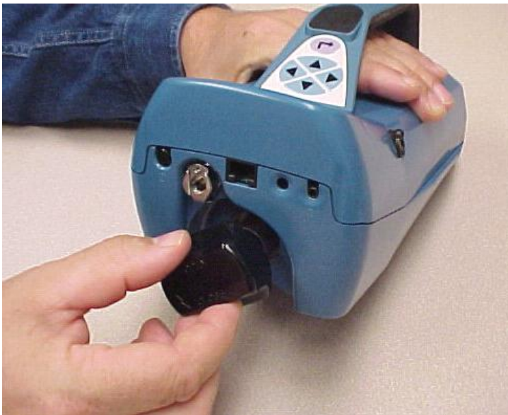
Figure 2-6: Insert Alcohol Cartridge into P-Trak Particle Counter
