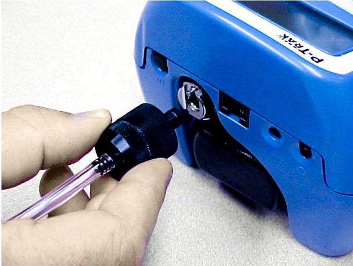
Figure 2-7: Insert Inlet Screen Assembly into Fitting
