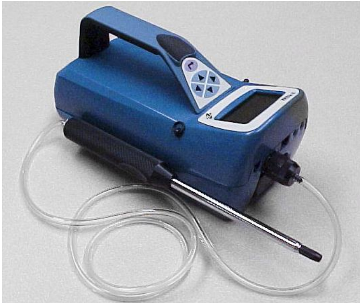
Figure 2-8: Slide Telescoping Probe onto Instrument Case
