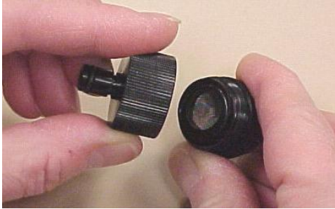
Figure 4-4: Re-assemble Inlet Screen Assembly
