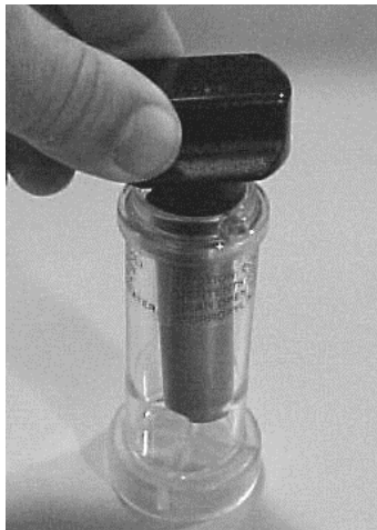
Figure 2-5: Insert Alcohol Cartridge into Fill Capsule
