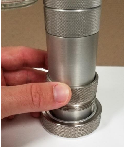
Figure 17: Unscrew the top knurled ring
