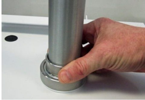
Figure 38: Secure inlet column to retainer ring
