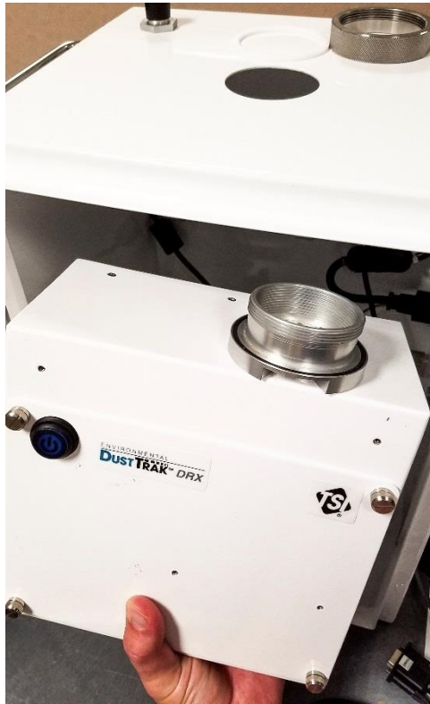
Figure 28: Removing the instrument from enclosure
