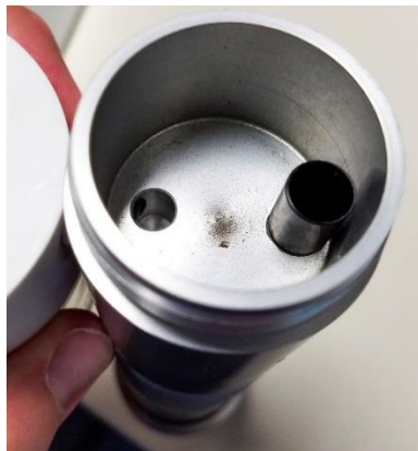
Figure 40: Cleaning near the water trap
