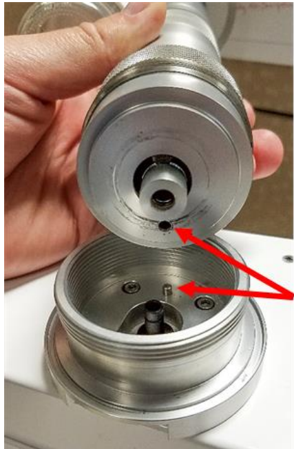
Figure 37: Aligning inlet assembly
