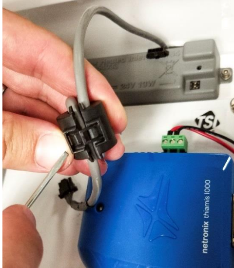
Figure 20: Removing ferrite clamp assembly
