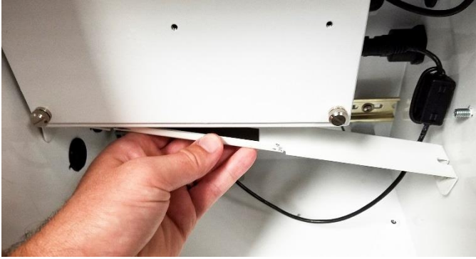
Figure 26: Removing instrument from mounting bracket
