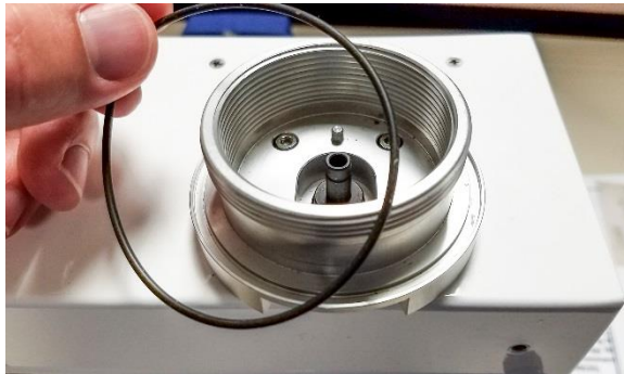
Figure 29: Removing rubber O-ring from mounting ring
