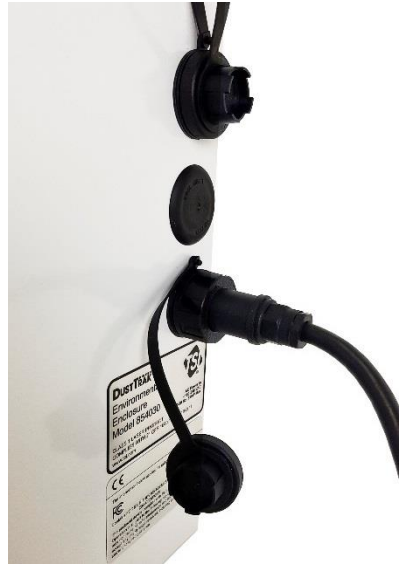
Figure 8: Connecting power cord
