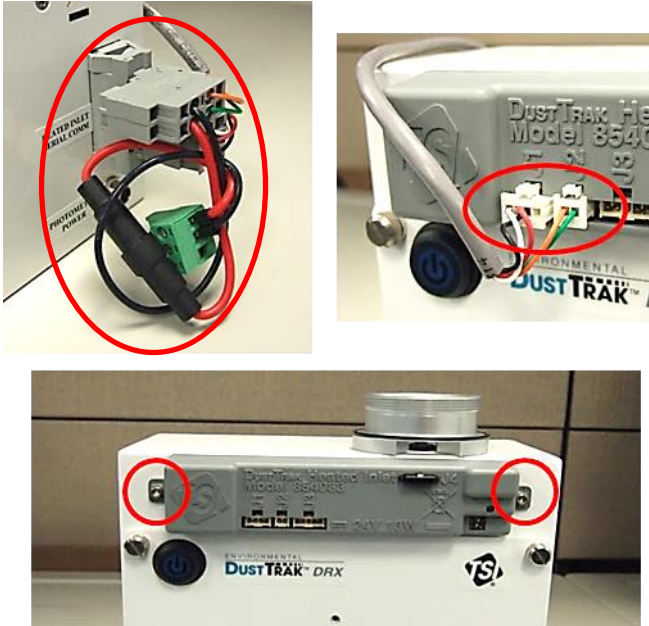
Figure 30: Removing cables and heated inlet controller
