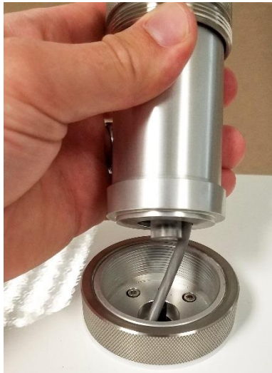
Figure 21: Pull heated inlet assembly up
