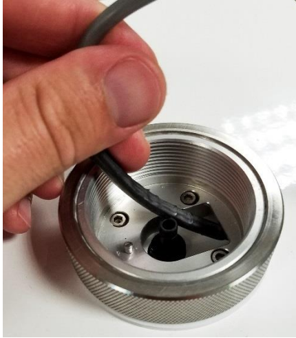
Figure 22: Removing heated inlet assembly
