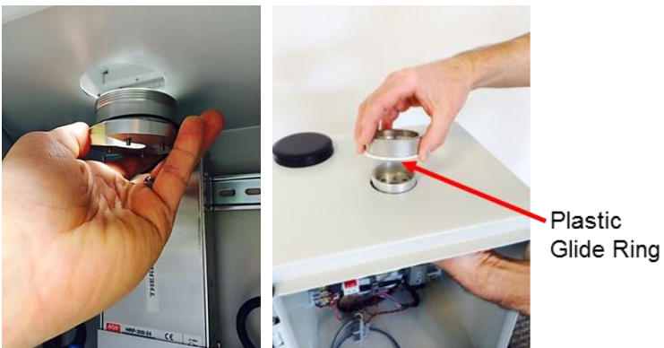
Figure 35: Secure retainer ring
