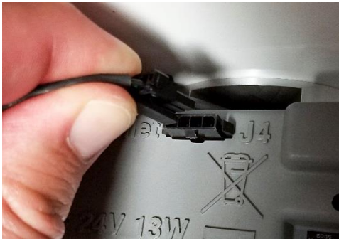
Figure 19: Disconnect heated inlet cable
