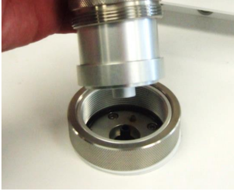
Figure 18: Remove inlet assembly
