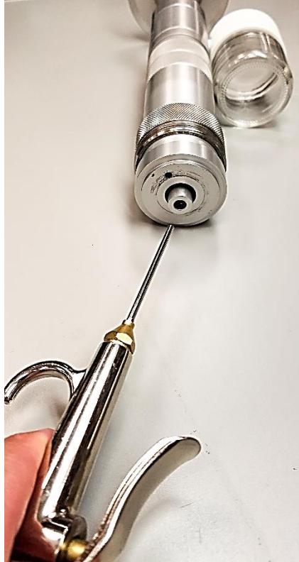
Figure 39: Blowing compressed air through the inlet
