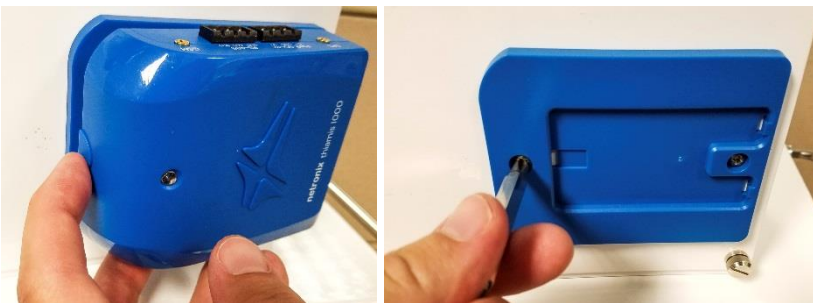
Figure 31: Removing Thiamis™ 1000 modem
