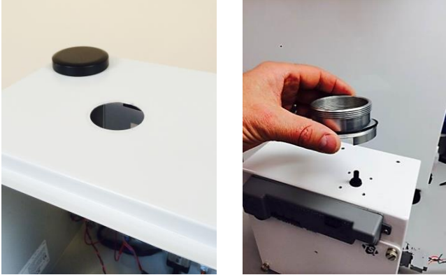
Figure 34: Remove mounting ring from photometer
